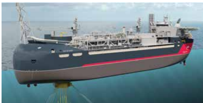
Illustration of the floating production storage and offloading (FPSO) unit
