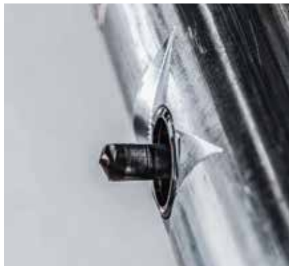
The Welltec Puncher 218 provides an e-line conveyed, non-explosive method for equalizing pressures between tubular strings.
