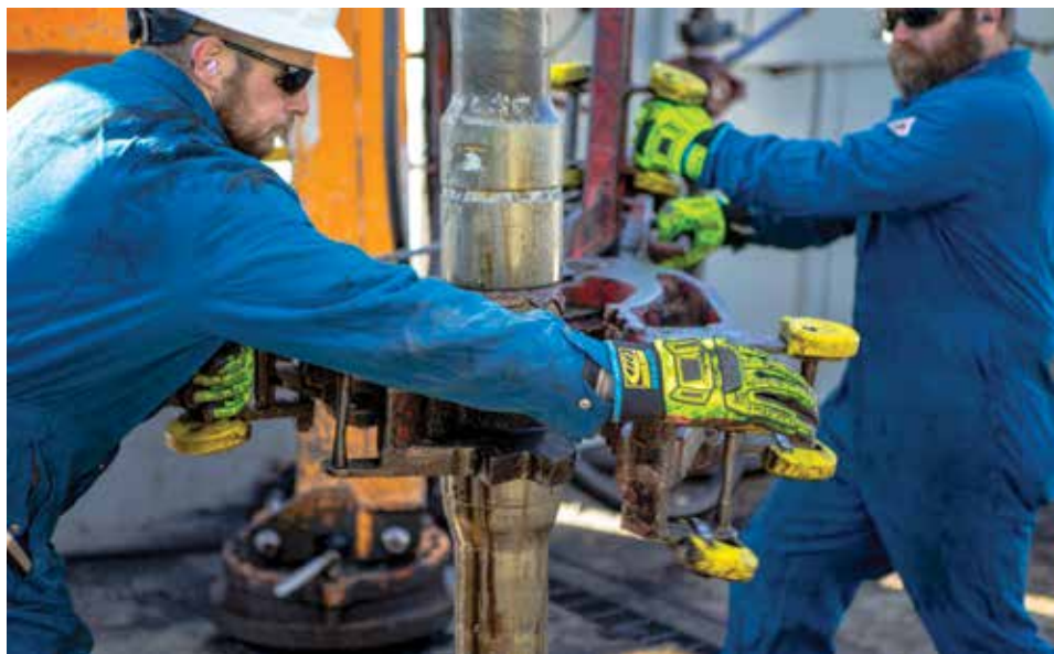
Righands connect drillpipe on Rig #45 in northeastern Pennsylvania for Southwestern Energy in October.
