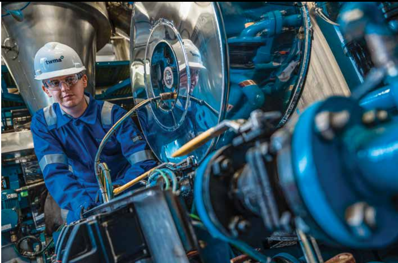
TWMA, a portfolio company of Buckthorn Partners, developed the TCC RotoMill, a technology that separates drill cuttings for recycling and reuse.
