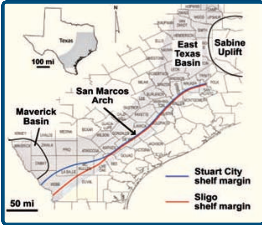
Overview reveals the known Texas extent of the Eagle Ford Formation with the major tectonic features affecting Eagle Ford deposition. (Unless otherwise note, illustrations from "Regional Stratigraphic and Rock Characteristics of Eagle Ford Shale in Its Play Area: Maverick Basin to East Texas Basin," by T.F. Hentz and S.C. Ruppel, reprinted with permission of the Bureau of Economic Geology)
