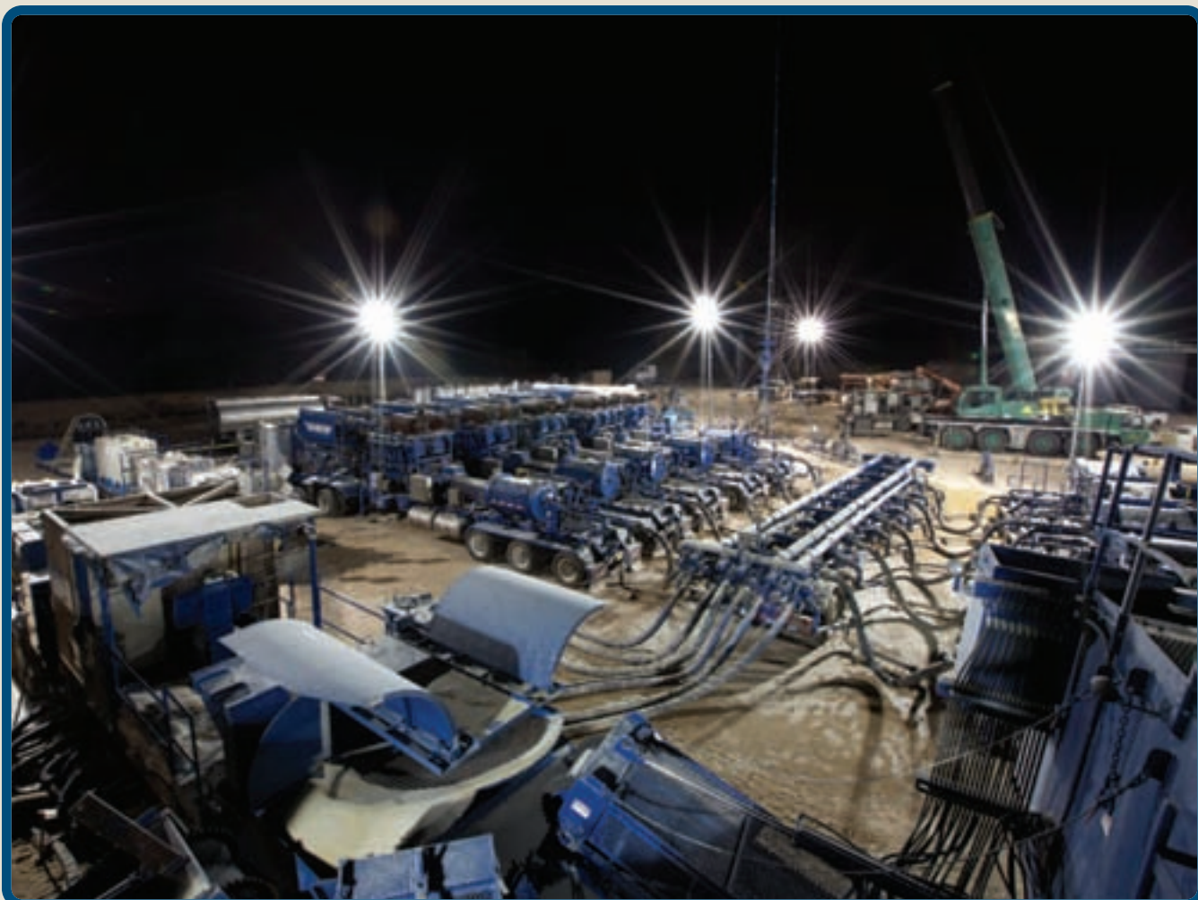
Schlumberger performs a HiWAY fracture stimulation job on one of BHP Billiton's Eagle Ford wells. (Photo courtesy of BHP Billiton)
