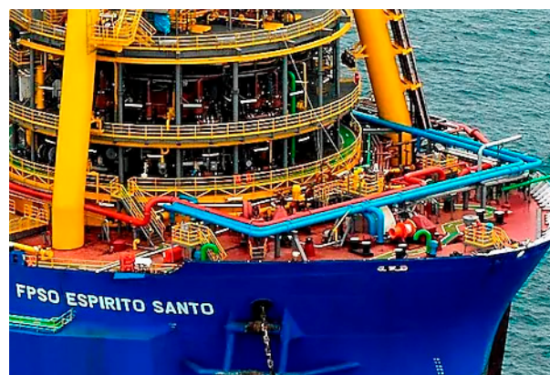
Shell’s FPSO Espirito Santo has a storage capacity of more than 2 MMbbl. (Source: Shell Brasil)
