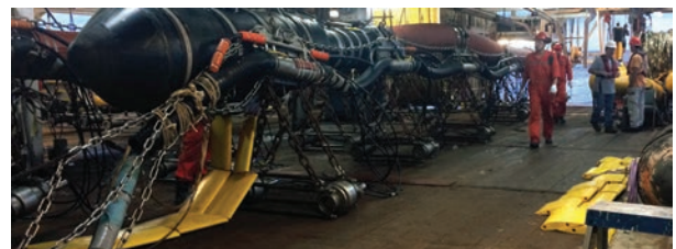
MacArtney's SailWing actuator is designed for correct positioning and stability of seismic survey arrays. (Source: MacArtney)
