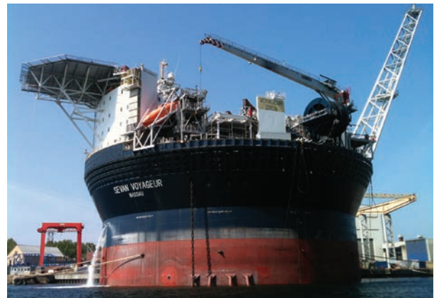
A Sevan cylindrical rig will be used on the North Sea field.
