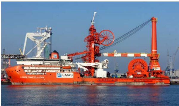
The Lewek Constellation pipelay vessel
