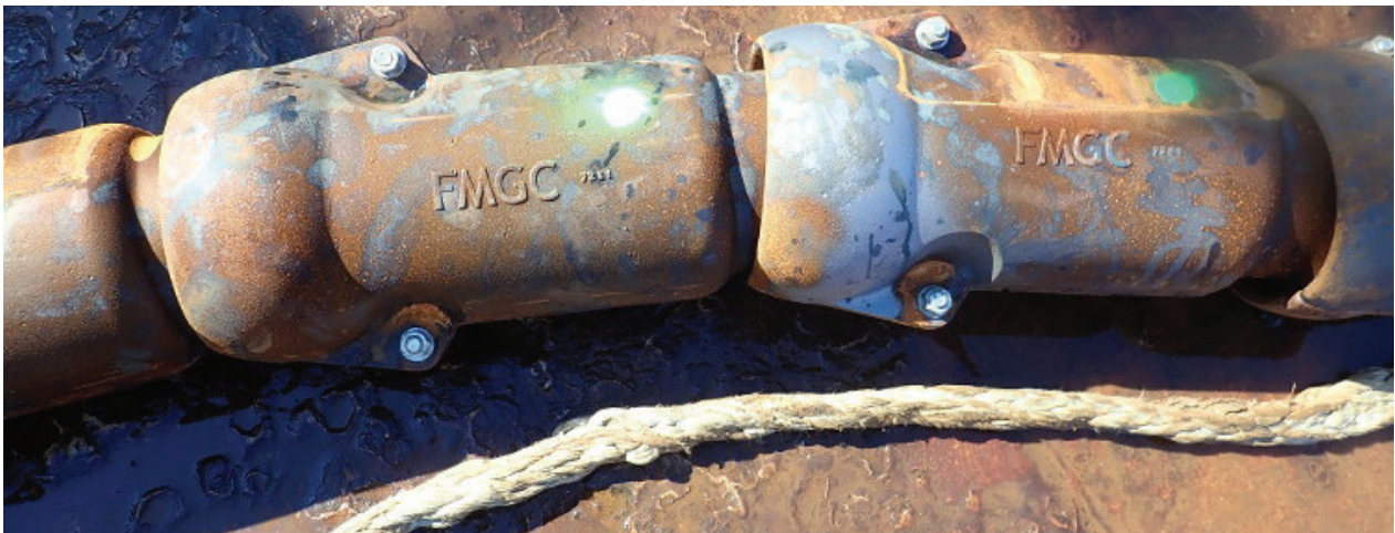
The shells stabilize and limit the curvature of submarine electrical cables. (Source: FMGC)
