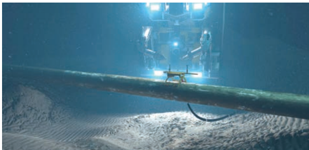
The Sea Turtle uses electromagnetic acoustic transducers to assess the plate or pipe condition of structures, pipelines, jumpers, flowlines and risers. (Source: Oceaneering)
