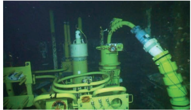
Trendsetter TC7 is used to connect the Mt. Providence subsea well to the Pompano template system. (Source: Trendsetter Engineering)
