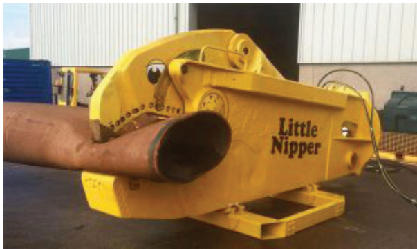
Little Nipper is a subsea cutting tool with a jaw capacity of 1.2 m in diameter (Source: JFO)
