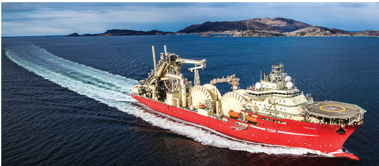
Skandi Recife can lay flexible pipelines in depths of up to 2,500 m. (Source: TechnipFMC)
