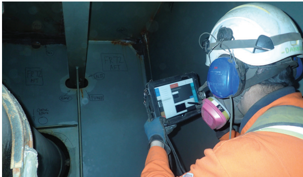
Pyxis helps assess structural integrity issues on FPSOs and FSUs. (Source: Marine Technical Limits)
