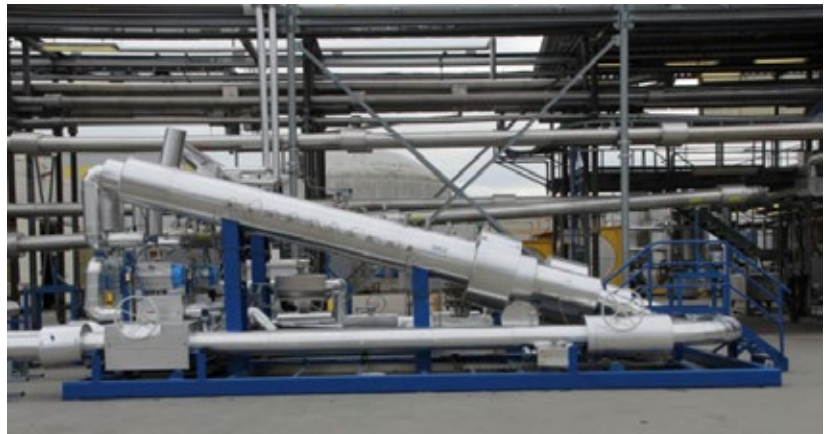
The full-scale and fully tested Dual Pipe Separator system separates the stream under flowing conditions without the pressure losses seen in a conventional system. (Source: Seabed Separation)
