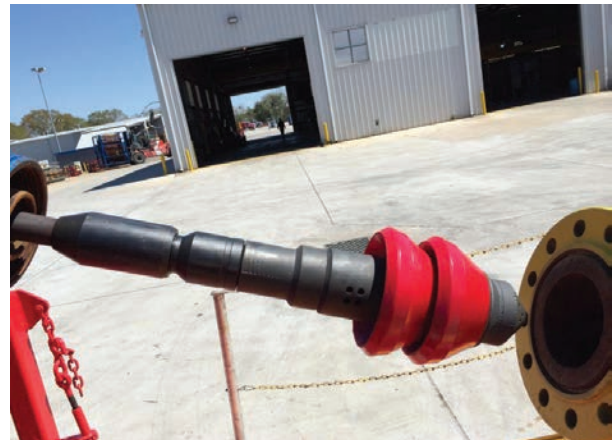
The CT-deployed CoilTac tool has been used to distances in excess of 1,219 m to remove paraffin, hydrate plugs, asphaltenes, scale and other blockages to the full ID of the pipeline. (Source: Superior Energy Services)
