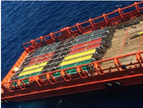
Dressed landing string joints, which were made up in a controlled environment onshore, arrived to the drilling vessel ready to be deployed. (Source: Landing String Solutions LLC)
