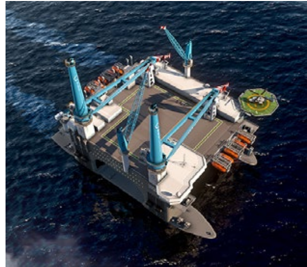
A photo illustration shows how the OOS Serooskerke and OOS Walcheren will appear. The two semisubmersible heavy-lift, construction and accommodation vessels are under construction. They will each be equipped with CCTV systems. (Source: O.O.S. International)
