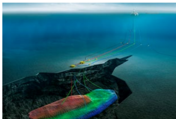
Fenja will be developed with subsea facilities tied in to the Njord platform. (Source: VNG)
