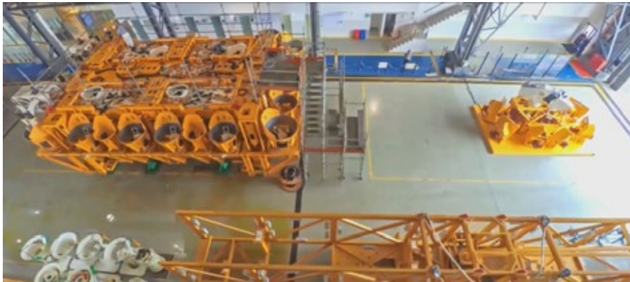
The compact manifold (right) is about one-quarter of its original size and half the weight with 70% fewer parts. (Source: TechnipFMC analyst day presentation)
