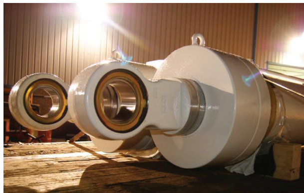
The locking mechanisms of subsea connectors use hydraulics to move locks into place and can stay locked for up to 25 years. They need to be fully functional to be unlocked at the end of this period. (Source: Apex Hydraulics)
