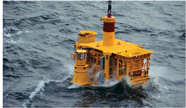
A subsea tree comprised of cost-efficient equipment components. (Source: Schlumberger)
