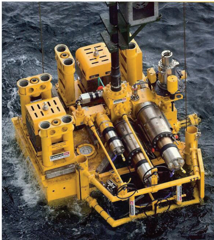
Cameron, now part of Schlumberger, delivered the first two all-electric Christmas trees to Total for installation on the Dutch K5F Field in 2008. (Source: Cameron)
