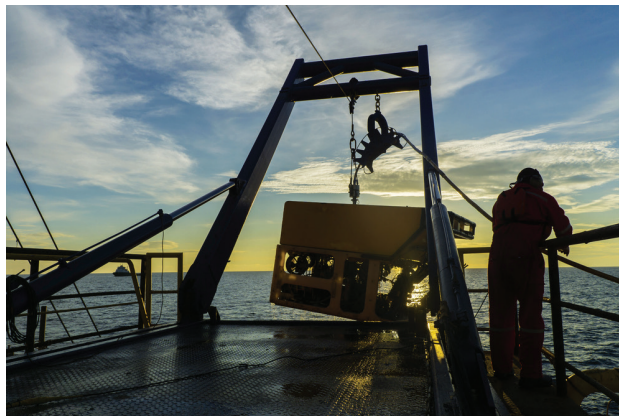
A worker recovers an ROV after inspecting an oil and gas pipeline. (Source: Karl Stury/Shutterstock.com)
