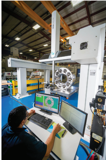
An H4 connector undergoes post-machining inspection. (Source: GE Oil & Gas)
