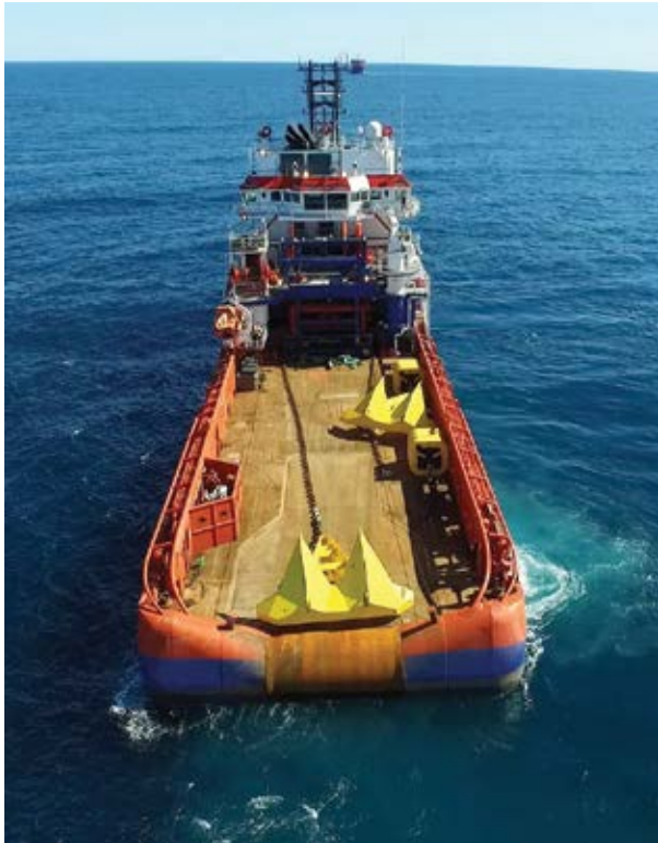
Twelve of Global Maritime's 20-tonne mK5 StevShark anchors from its sister company Vryhof were used as part of the Australian semisubmersible mooring solution. (Source: Global Maritime)
