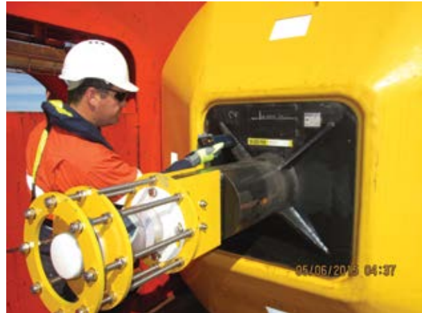
A newly patented radio-frequency identification marking system helps ensure complete traceability and an accurate usage history of the equipment. (Source: Global Maritime)
