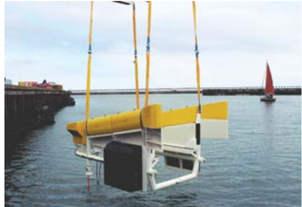
Osbit’s subsea garage is lowered into the water during an equipment trial. The equipment was designed for U.K.-based Modus for its Saab Sabertooth hybrid AUV. (Source: Osbit)
