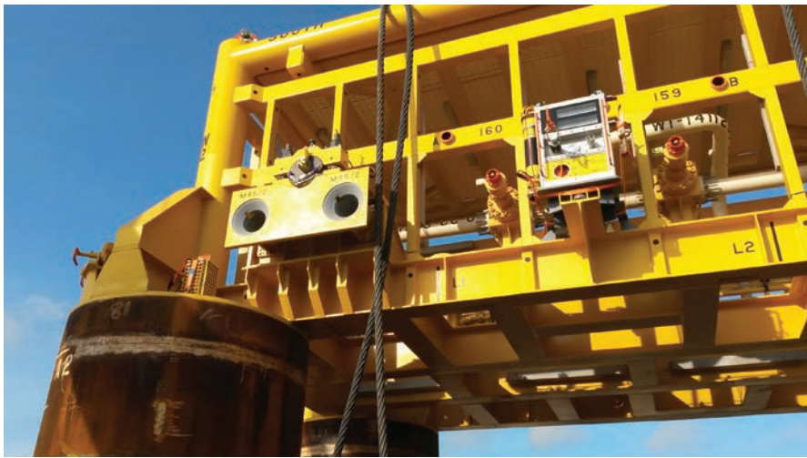
Ashtead's Deflection Monitoring System (DMS) is shown during mobilization. (Source: Ashtead Technology)
