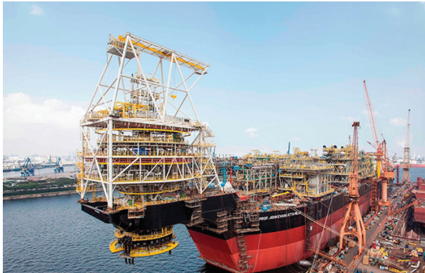
The Prof. John Evans Atta Mills FPSO vessel will produce and store oil from the TEN oil fields offshore Ghana. (Source: Tullow Oil)
