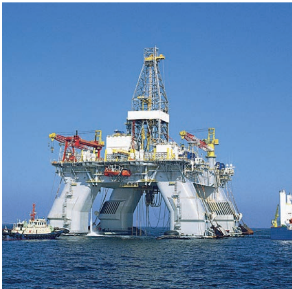
Transocean's Deepwater Nautilus semisubmersible unit drilled the Appomattox discovery well for Shell in 2010.
