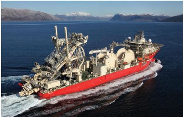
The Deep Energy pipelay vessel will be put to work on Bahr Essalam 2.
