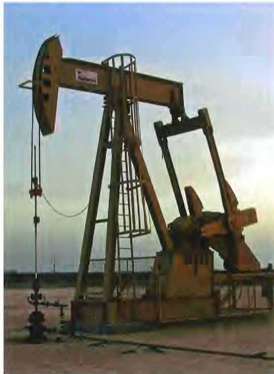
Maximizer pumping units are applied frequently in West Texas oil fields. (Photo courtesy of Weatherford)
