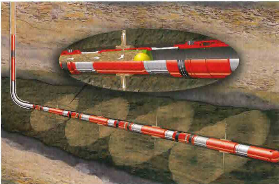
Delta Stim Plus 20 completion service provides operators new options for completing horizontal multizone well bores to enable highly accurate placement of fractures with minimal or no intervention. (Illustration courtesy of Halliburton)
