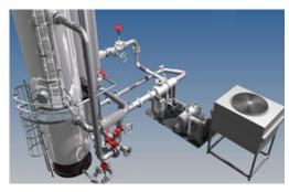
The companies said that the HMT module also helps to improve fractionation since it is incorporated into the stripping section of the fractionation column. This provides external heat input across the entire stripping section to generate stripping vapors which promotes mass transfer contact within the module.
