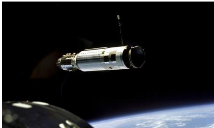
The Agena Target Vehicle is seen from the Gemini 8 spacecraft in a photo taken by astronaut David Scott during rendezvous on March 16, 1966. This was the first time two spacecraft successfully docked, which was a critical milestone if a mission to the Moon was to become a reality. (Source: NASA)
