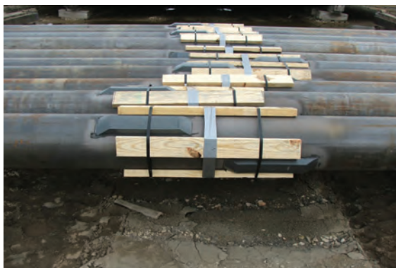
FIGURE 6. Field-molded stand-offs help ensure complete cement distribution and bonding.
