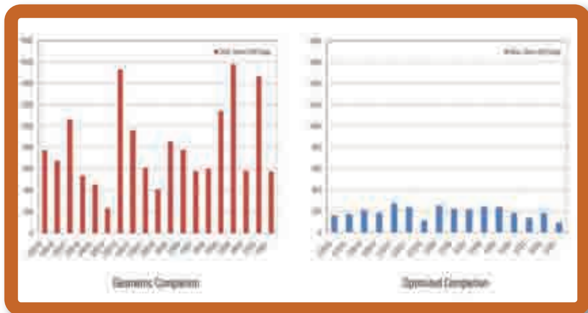
Figure 3. This image compares the maximum and minimum stress perforation clusters across the entire well bore. Using an optimized completion resulted in lower differential stresses gave the completions team confidence in increasing the stage length. This resulted in a reduction of three stages and stimulates a greater percentage of perforation clusters. (Image courtesy of Schlumberger)
