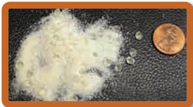
Multiple particle sizes of BioVert NWB diverter help achieve bridging for a highly effective seal and diversion to another designed zone. (Image courtesy of Halliburton)
