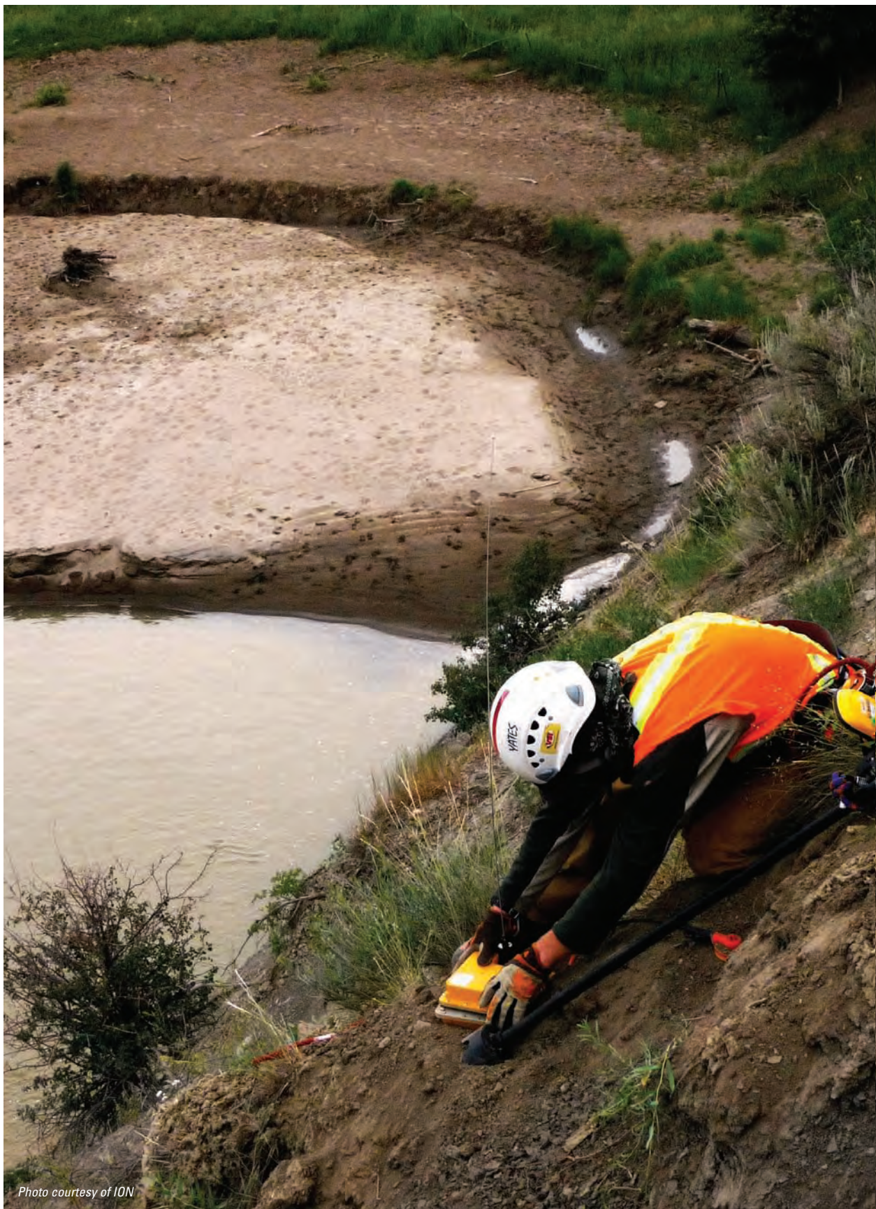
FIGURE 1. Experienced mountaineers carefully position remote FireFly sensor packages in rugged terrain that would prove extremely challenging for conventional cabled sensor networks.
