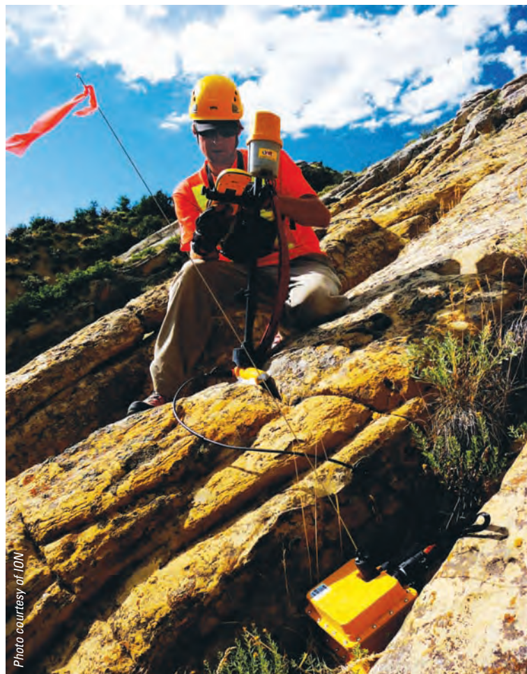
FIGURE 2. Remote sensor packages contain triaxial VectorSeis solid-state geophones and a two-way radio transceiver with GPS capability.
