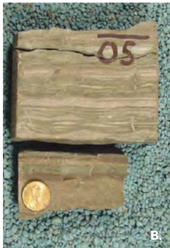
Sanish Sandstone: Core photographs representative of "Sanish" sandstone from the Raymond T. Duncan #1 Rose (Section 2-153n-94w). A: Medium-brown, highly burrowed siltstone to very fine-grained sandstone characteristic of the "Sanish" sand (depth – 10,601.3 ft). B: Characteristic apple green and tan interbedded sequence of the Three Forks Formation (depth – 10,605 ft). Adapted from LeFever & Nordeng, North Dakota Geological Survey, Bakken core short course, July 7-8, Denver, Colo.
